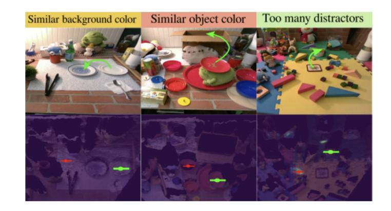
Typical Failure cases occur when the background color is similar to the pick or place object. Or one of a few distractors has a very bright color or similar colors.
