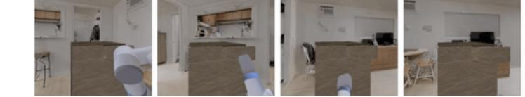
In addition, we test GenAug on a new task "close the top drawer" with a fetch robot. In particular, We tested on 100 unseen backgrounds using iGibson rooms and observed GenAug is able to achieve 60% success rate while policy without Genaug is only 1%.
